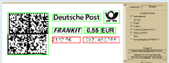
Figure 4: Prepaid FRANKIT franking with partially displaced but read data matrix code and two unrecognized characteristics
