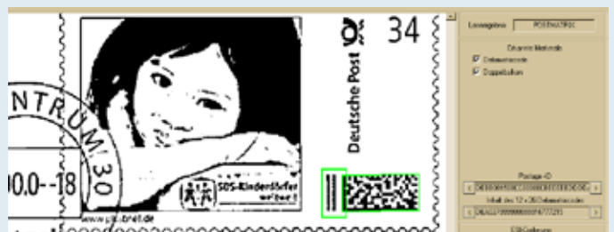
Figure 5: Read post matrix code on a "Plusbrief" (envelope with a printed postage stamp on it)
