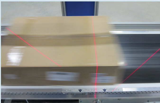
VIPAC enables the reliable detection and discharge of damaged cartons during the conveying process
